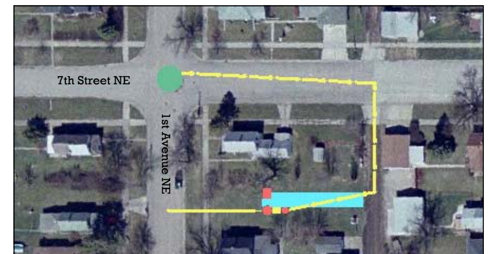
New gravity sewers and a forcemain (yellow lines) will lead to the new lift station (above ground structures in red). An access road (light blue) will be constructed as well.
